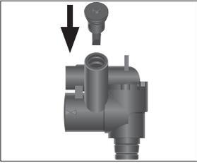
► Fit the air intake pipe.
